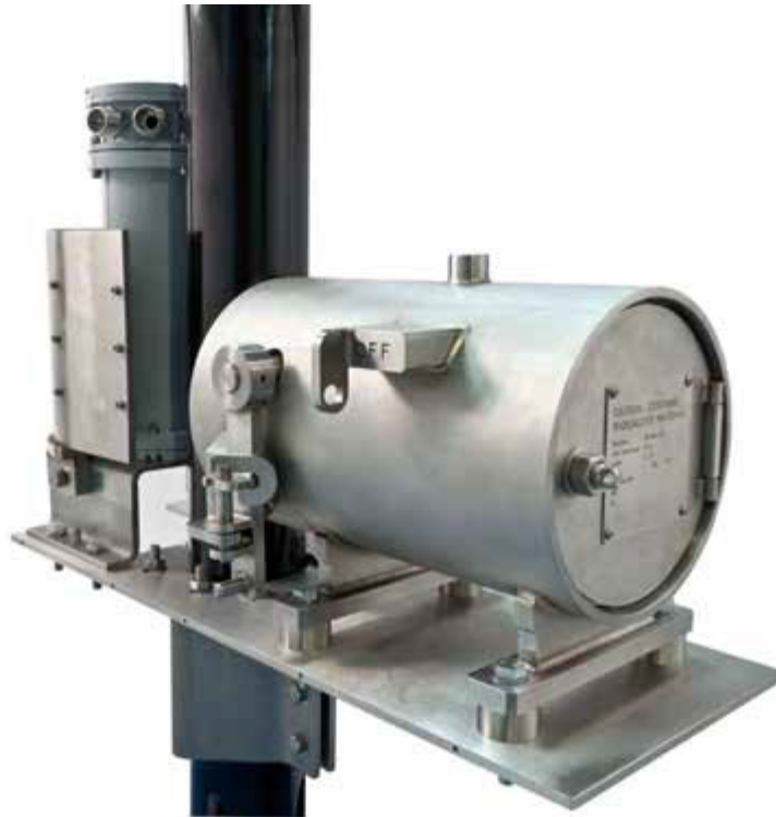
Neftemer meter clamped-on to a 4in flowline
